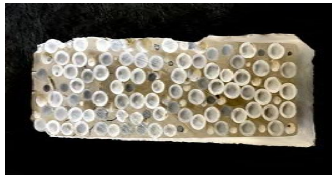
Figure 5: Vertical section of the glass cylinder filled with polydisperse glass beads (50% of 8 mm, 33% of 12 mm and 17% of 16 mm) after mortar infiltration and setting.
