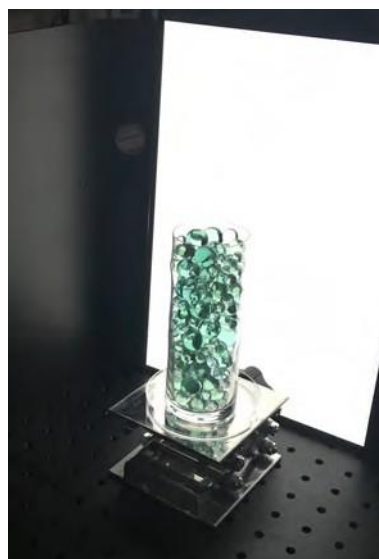
Figure 3: Optical setup for mortar injection in a cylinder filled with glass beads.
