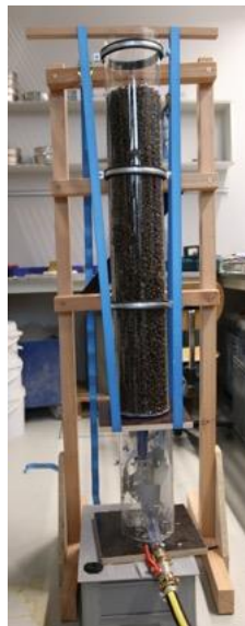
Fig. 7.4 – Picture of infiltration setup from bottom.
