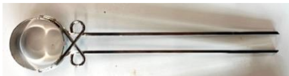
Fig. 9.3 – Picture of the Le Chatelier ring
