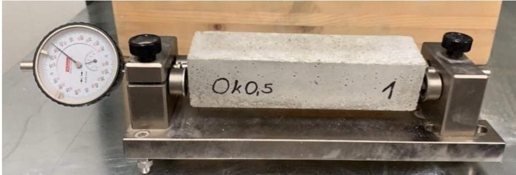
Fig. 9.1 – Setup for concrete sample length measurement
