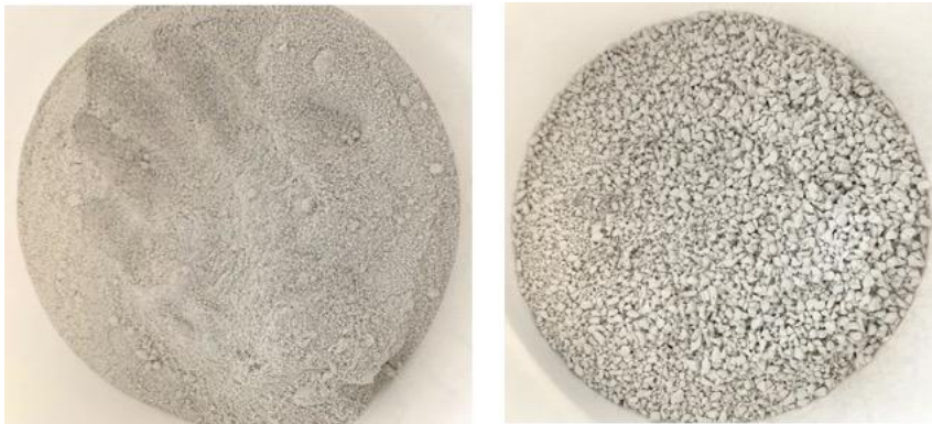
Fig. 9.2 – Pictures of obtained fine-grained plaster (left) and coarse-grained plaster (right)
