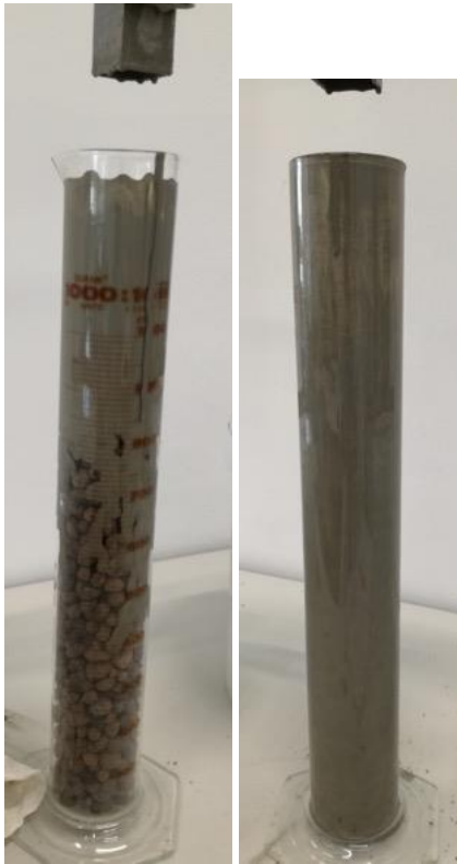
Fig. 7.1 – Pre-wetted large LECA beads infiltrated by a cement slurry placed from top. Infiltration was successful as all beads are surrounded by cement.
