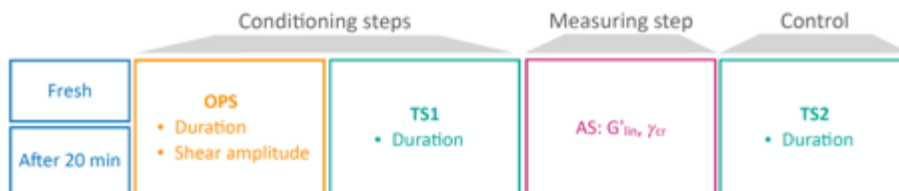
Fig. 3.3: Sketch showing the complete protocol on fresh and after 20 min samples. An oscillatory pre-shear (OPS) of \gamma = 100\% is applied in the conditioning step of the measurements.
